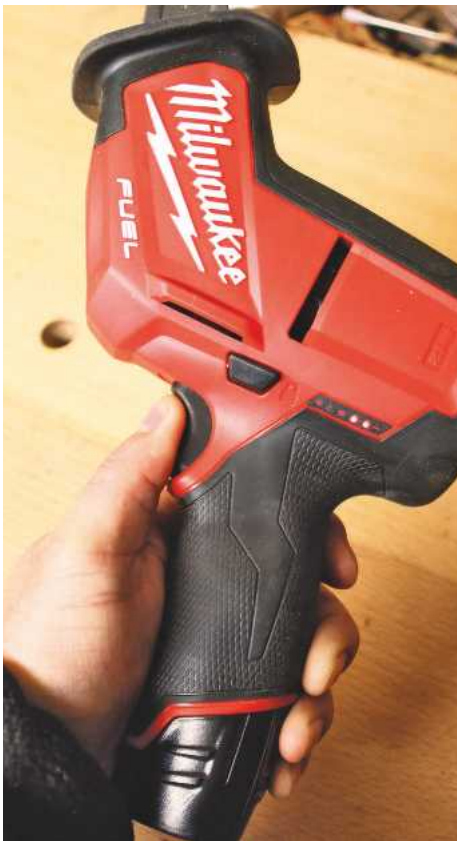
▲ A touch on the variable-speed trigger illuminates lights on the tool to show the battery status
